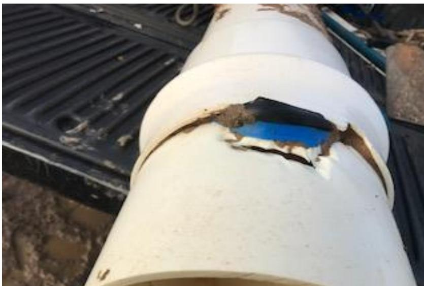
A further two blowouts associated with air getting trapped in the system following long periods of non-operation. This has been overcome by re-programming the startup intensity of the pressure pumps and with the addition of 4 more air valves to allow release of trapped air.
